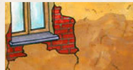
1. Plaster damaged by water and salts. Analyze the causes and assess the extent of the problem.
